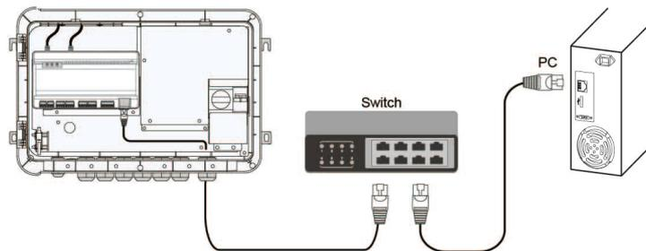
figure 5-2 Connection to PV background system
