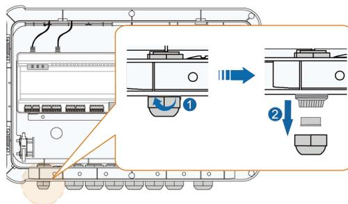
**step 4** Lead the cable through the nut, the waterproof plug and the waterproof terminal, and connect it to the interface on the master node of EyeW485. Adjust the cable and secure the waterproof terminal.
