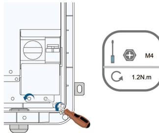
**step 2** Unscrew the "PLC" waterproof terminal at the bottom of COM100.
