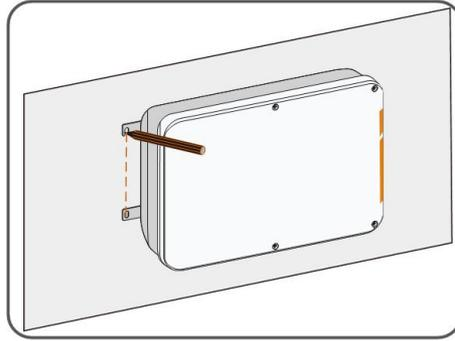
**step 3** Drill the holes with a drill according to the marks made before.
