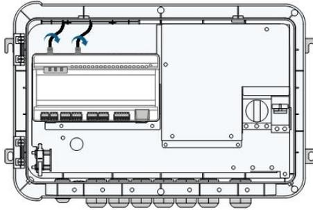
**step 3** Loosen the "RF" waterproof terminal on the bottom of the COM100.
