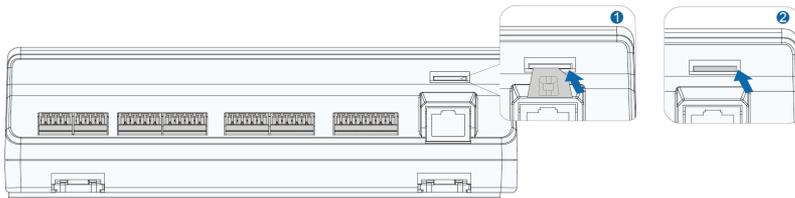
**step 3** Turn the power switch inside the COM100 to "OFF"
