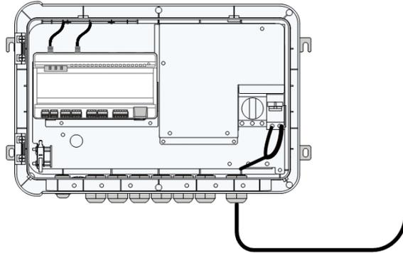
**step 3** Strip and connect the cable to the corresponding terminal inside the COM100.
