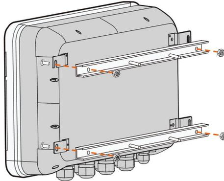
**step 2** Fix the mounting-brackets with the clamps by using the nuts.
