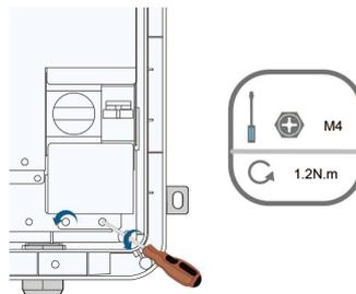
**step 2** Loosen the "AC (100~277V)" waterproof terminal, and insert the external power supply cable through the waterproof terminal into the corresponding terminal of the miniature circuit breaker inside the COM100.
