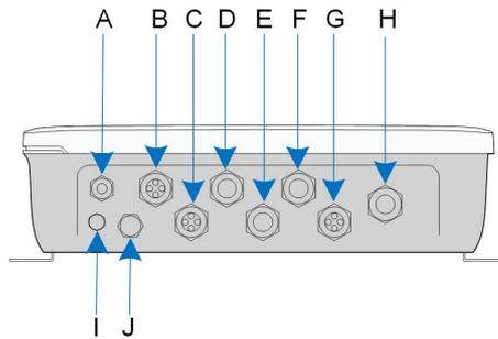
figure 5-1 Waterproof terminals on the bottom of COM100
