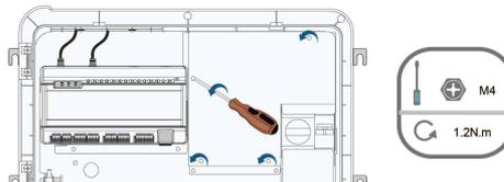
**step 2** Use screws to fasten the PCB.
