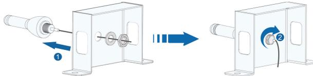
**step 3** Remove the nut and waterproof plug from the COM100 RF waterproof terminal.
