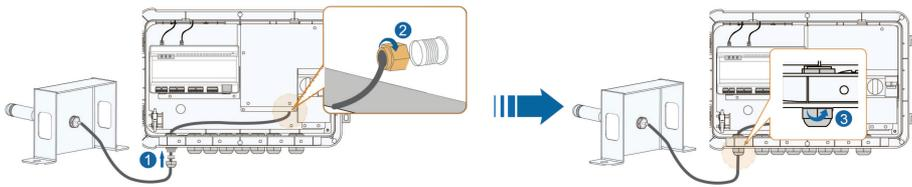
**step 5** Fix the antenna support to the mounting plane or the pole.
