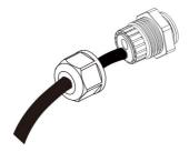
step 4 Plug the wires into terminals A2 and B2 on the inverter without tool tightening.
