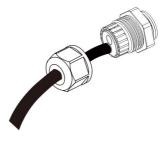
step 3 Remove the cable jacket and strip the wire insulation.
