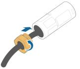
step 2 Put the locking ring into the housing.
