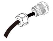
step 3 Remove the cable jacket and strip the wire insulation.
