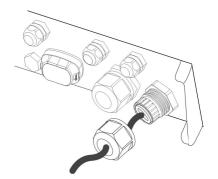
step 5 Loosen and remove the screw sets on the **BAT +** and **BAT-** terminal blocks. Fasten the cables to the corresponding terminals with a torque of 2.5 N.m.
