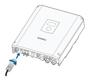
step 6 Connect the other ends to the emergency loads. Pull all the lines outward to check whether they are firmly installed.
