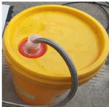
figure 4-4 Temporary liquid accumulation buckets
