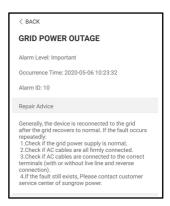
figure 7-9 Detailed Fault Alarm Information
