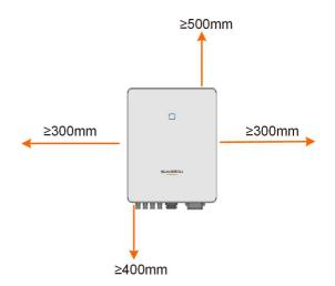
In case of multiple inverters, reserve specific clearance between the inverters.
