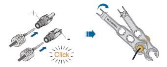
step 5 Check for polarity correctness.
