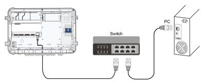
figure 4-2 Connecting to Background of PV System
