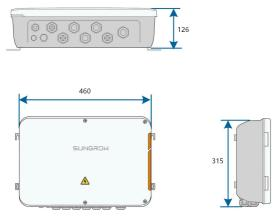
figure 2-2 Dimensions of COM100 (mm)
