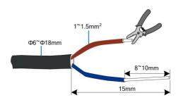
step 3 Insert the stripped DC cable into the port "24V OUT +" and "24V OUT -" of the Logger1000.
