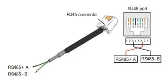
table 4-3 Correspondence Between Wire Colour and Pin of RJ45 Connector
