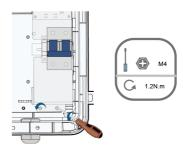
**step 2** Loosen the "AC (100 – 277V)" waterproof terminal, and insert the external power supply cable through the waterproof terminal into the corresponding terminal on the miniature circuit breaker inside the COM100.
