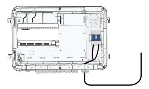
step 3 Strip and connect the cable to the corresponding terminal inside the COM100.
