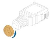
**Step 2** (Optional) Remove the inner sealing ring if the cable diameter is 19 mm–25 mm. Otherwise skip this step.
