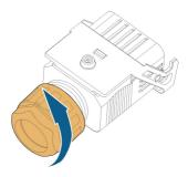
Step 2 Take out the spring-loaded terminal from the housing.
