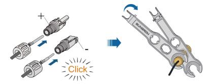
Step 5 Check for polarity correctness.
