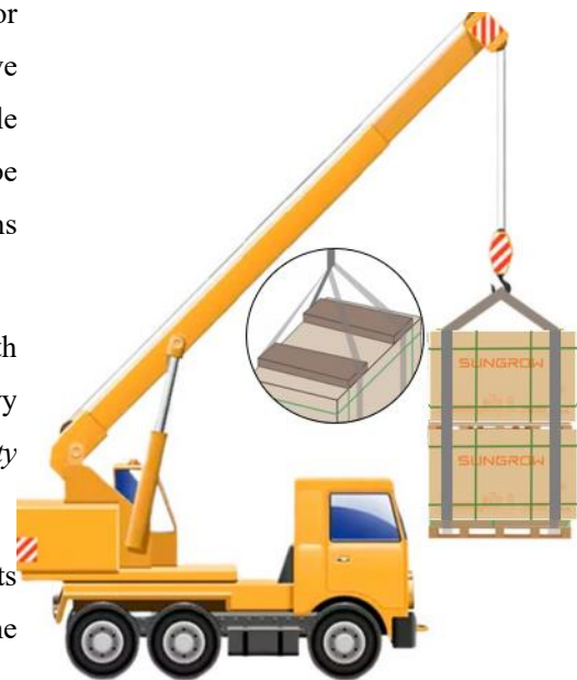
Fig. 3 Diagrammatic sketch of lifting the Modules
