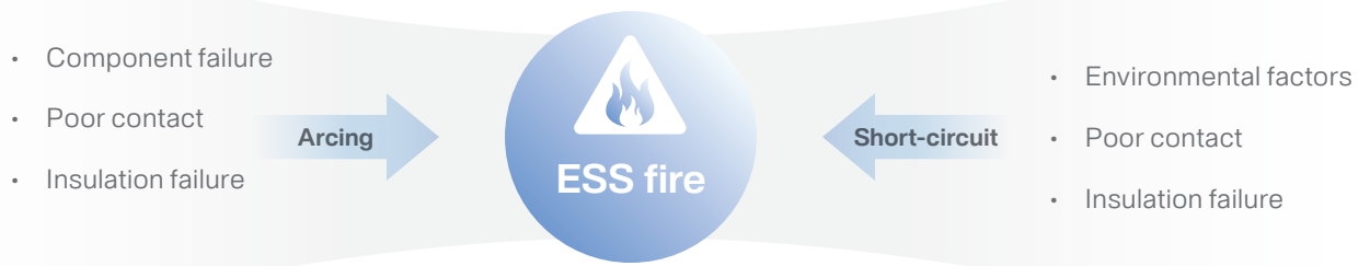
Figure 6: Analysis of causes of ESS fire accident
