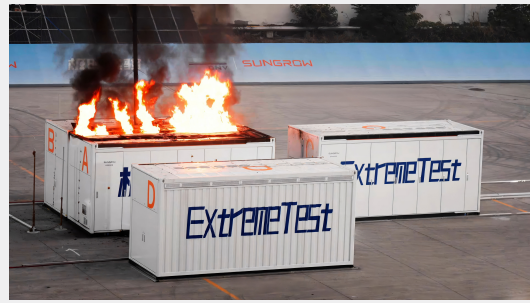
Figure 37: On-Site Large-Scale Burn Test of PowerTitan
