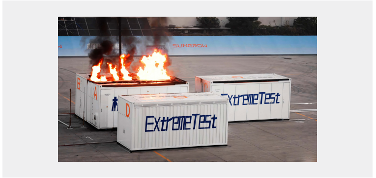
Figure 37: On-Site Large-Scale Burn Test of PowerTitan
