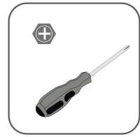
Phillips screwdriver (M4, M6, M8)
