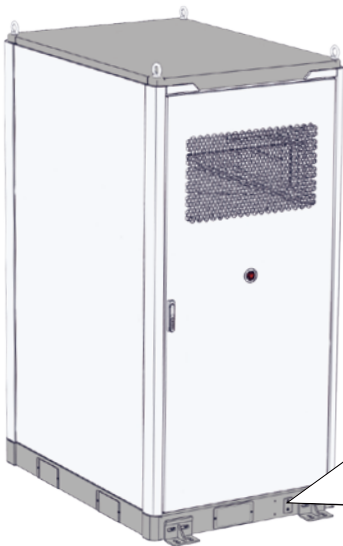
Option 2: Grounding flat steel
