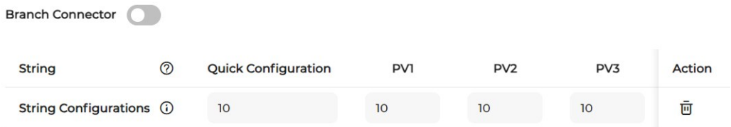
Figure 4-7 Strings have the same number of modules
