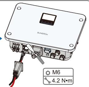
\*Gently pull the cable backward to ensure firm connection.
