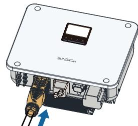
\*Gently pull the cable backward to ensure firm connection.
