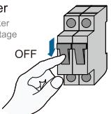
\*When the battery has no switch, a DC breaker should be added.
