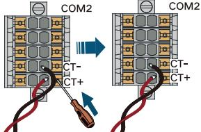
\*Please insert CT+ and CT- into positions 9 and 7 of the signal plug-in connector respectively.
