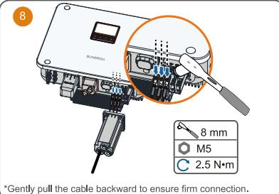
\*Gently pull the cable backward to ensure firm connection.
