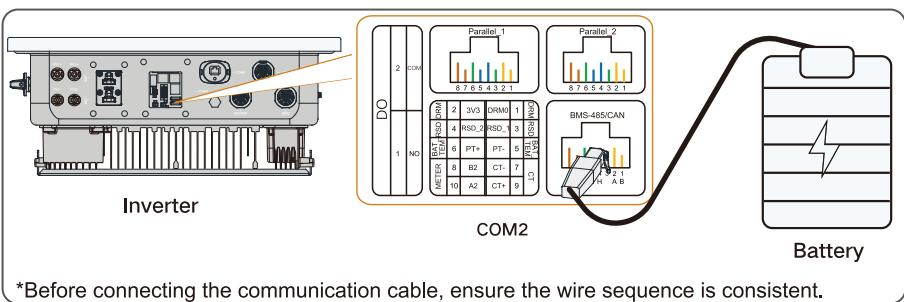
\*Before connecting the communication cable, ensure the wire sequence is consistent.
