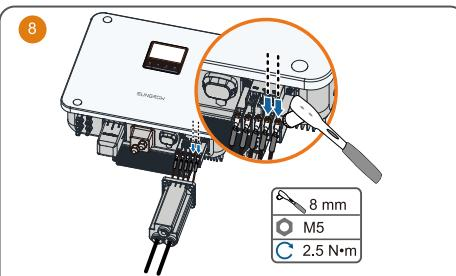
\*Gently pull the cable backward to ensure firm connection.
