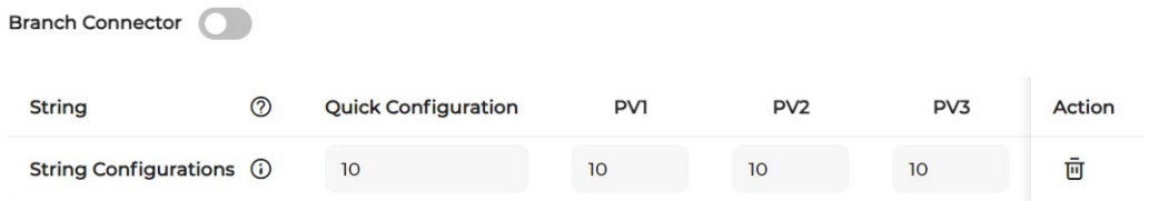
Figure 4-7 Strings have the same number of modules
