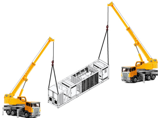
Figure 5-2 Lifting of two cranes
