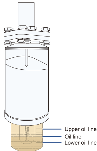
Figure 6-2 Fit the Oil Cup
